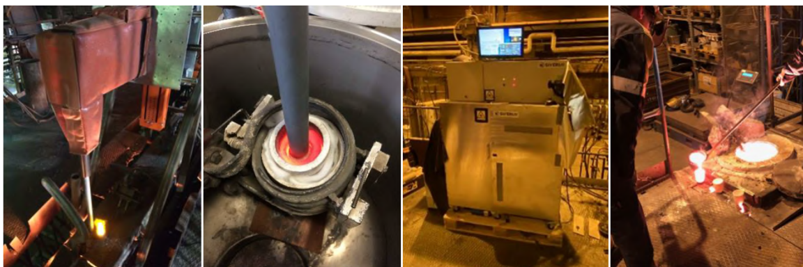
Figure 1. Examples of installations for slag analysis
