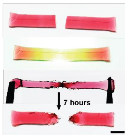
Figure 1: The phenomenon shown in four steps. First two parts, second irradiation of the interface, third the adhesion and pulling, fourth splitting of the sample after 7 hours.
