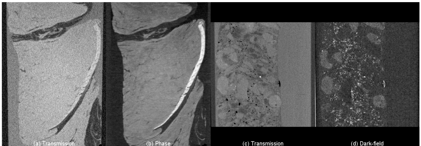
Fig. 1: Lateral slices from reconstructed tomography data sets of a piece of pork (a and b) and a sausage (bratwurst) filled with cheese and bacon (c and d). Both samples were placed in a cylindrical plastic tube filled with ethanol. The pork sample was additionally submerged in a water container (to reduce beam-hardening and phase-wrapping artefacts). A clear improvement in contrast is seen in the phase-contrast image (b) compared to the transmission image (a). In the case of the sausage sample, the dark-field image provides the most useful complementary information: While some areas in the transmission image (c) have nearly the same gray values, the contrast between the same areas in the scattering-based dark-field image (d) is much more pronounced.
