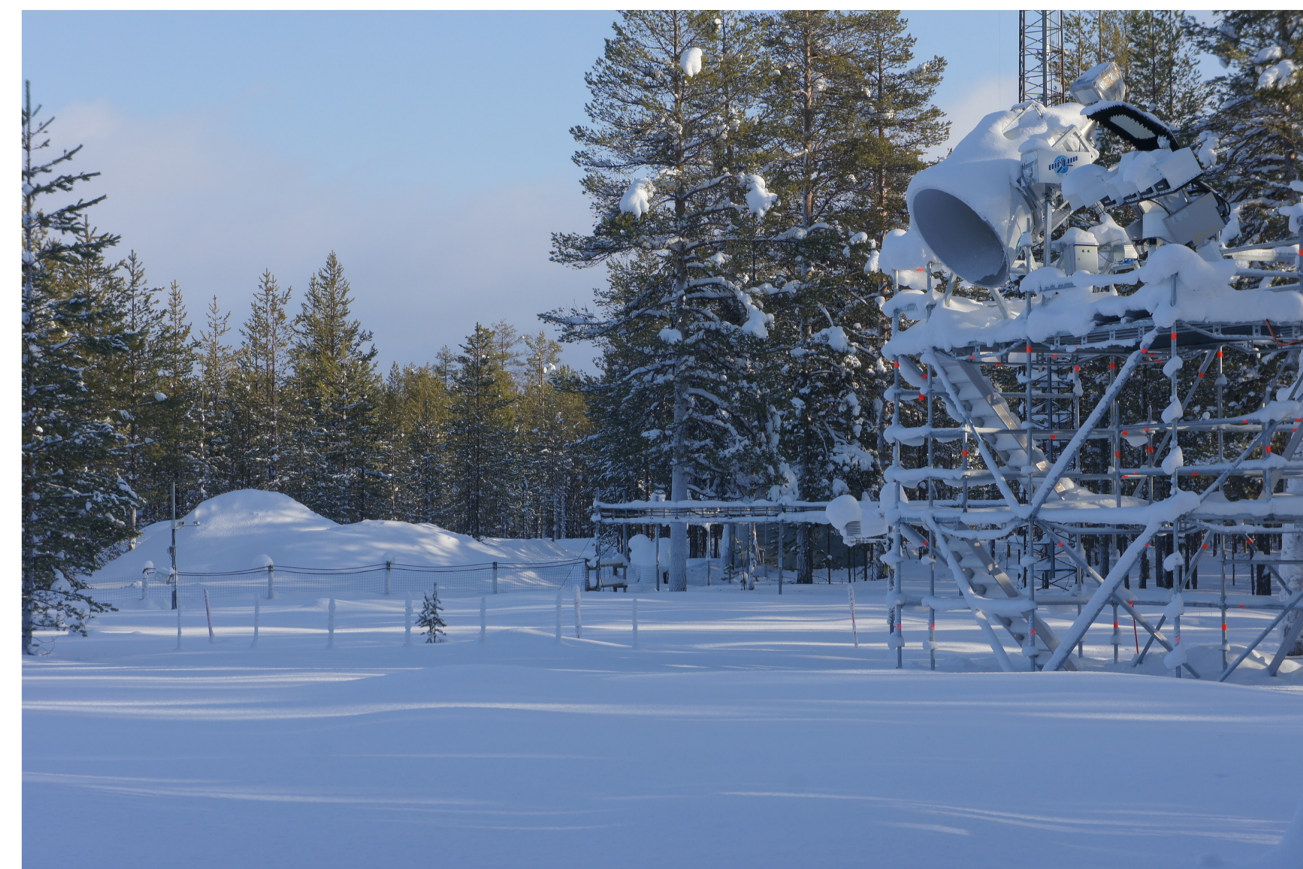
Figure 1: ELBARA-II measuring the upwelling brightness temperature at IOA site, located in Sodankylä, Finland. Photo: C. Mätzler, 2011
