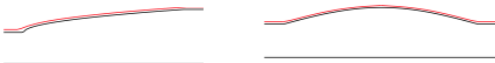
Figure 2: Reconstruction of two slowly varying waveguides. In black, the initial shape, in red, the reconstruction slightly shifted for comparison purposes.
