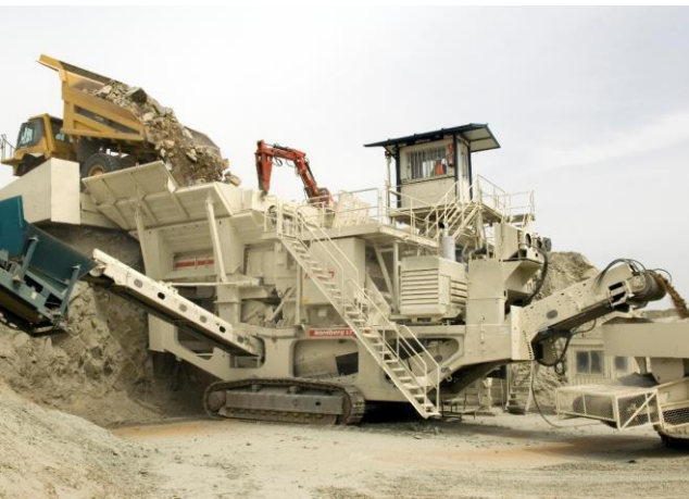
Lokotrack LT140 Jaw width 1400 mm, rock size < 900 mm
