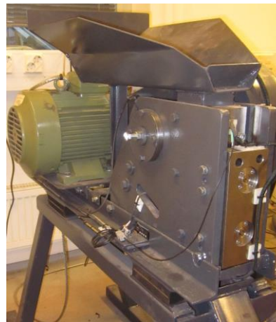
Laboratory crusher C7 Jaw width 70 mm
