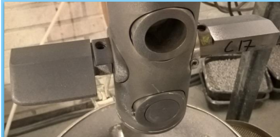
Slurry-pot with dry granite bed (Dry-pot)
