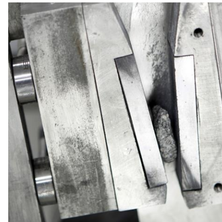
Dual pivoted jaw crusher Jaw width 25 mm
