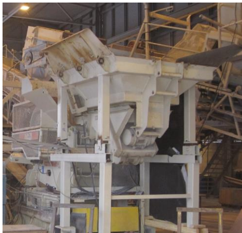
Metso C80 jaw crusher Jaw width 800 mm
