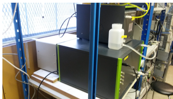
Figure 1. Setup showing the “sampling box” (in white) deployed in front of a PSM-CPC system (Airmodus A20).
