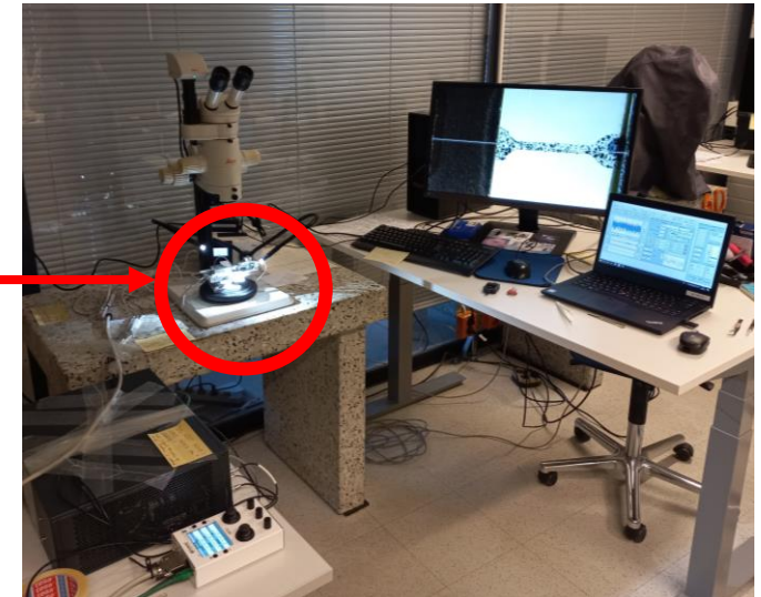
Loading under optical microscope: specimen deformation tracking with Digital Image Correlation
