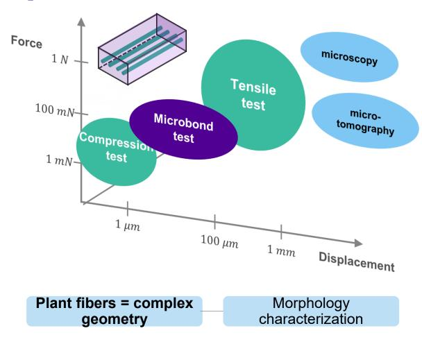
Fibers  $\sim$  transversely isotropic  $E_L/E_T$  ratio = high  $E_L o$  tensile testing  $E_T o$  transverse compression
