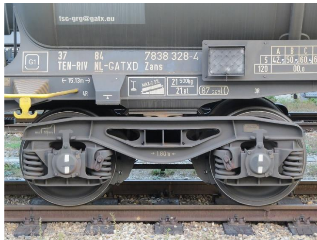
Figure 1. Typical Y25 freight bogie with coiled spring primary suspension and a lenoir link.
