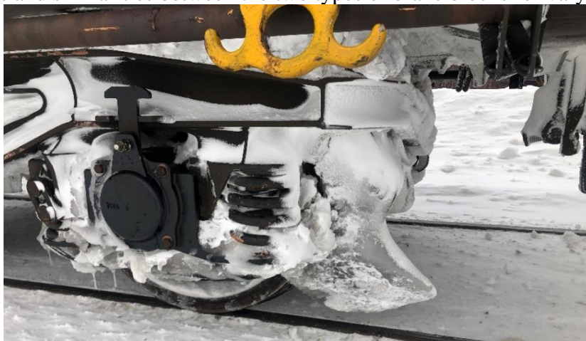
Figure 1. Example of build-up of ice and snow in bogie during winter conditions
