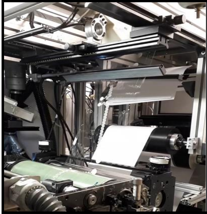
R2R printing of stretchable epidermal printed conductors
