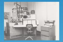
• JEM 200A transmission electron microscope
